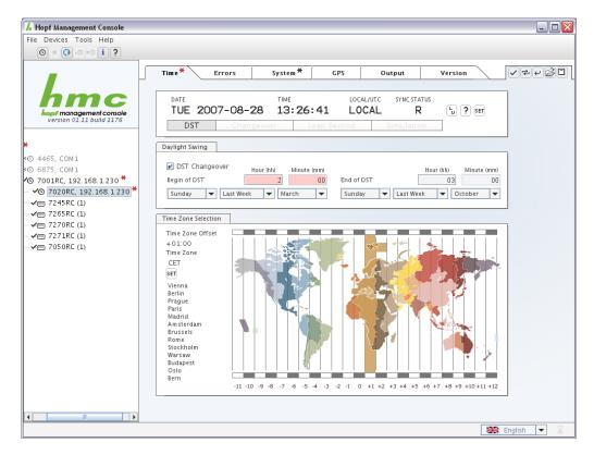
An example of an invalid input in the tab area *Time*. The *System* tab holds a black asterisk, indicating a value change. The device tree only shows a red asterisk which implies a value change anyway.
