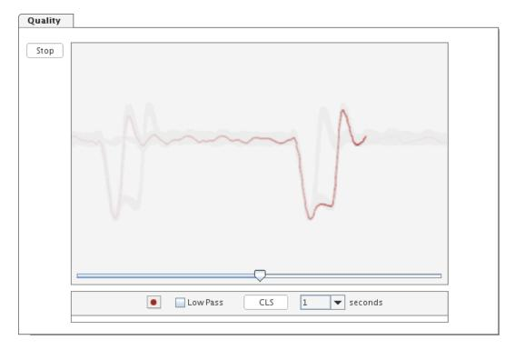
This signal, generated and emitted via radio in Braunschweig, Germany, transmits bits of information encoded as shorter and longer (typically 100ms and 200ms) signal level drops. The falling flank of these level drops signifies the exact second change. The Image shows more or less the ideal case of such a signal that is realized by connecting the DCF77 input to the DCF77 simulation output of another device, instead of to an antenna.
