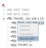
Recording can be started only for already connected GPS devices, all information is logged into a file and is visualized human readable in a dialog.
