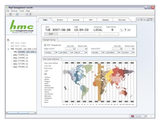
On top and to the right in the configuration view, there is a small tool bar for reading and setting device properties, as well as for loading and saving complete configurations.
