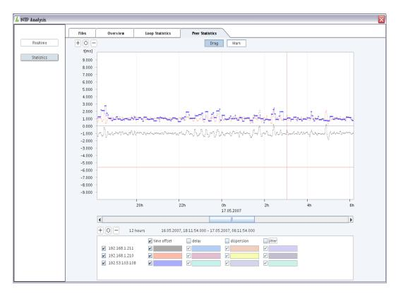
In the *Peer Statistics* area, the active peerstat files' content is displayed. Its handling is very much that of the *Loop Statistics* area, with a few differences:
